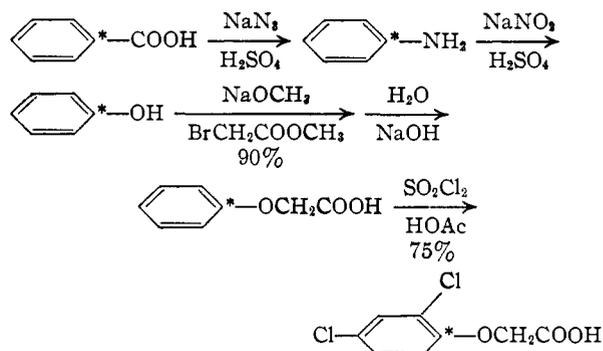
The concentration of the sulfuric acid employed in the Schmidt reaction with benzoic acid plays a significant role in determining the yield of aniline. In Table I are summarized the results observed with 96–100% sulfuric acid; under comparable conditions with 75% sulfuric acid, the yield of aniline is reported to be only 15%.<sup>4</sup>
