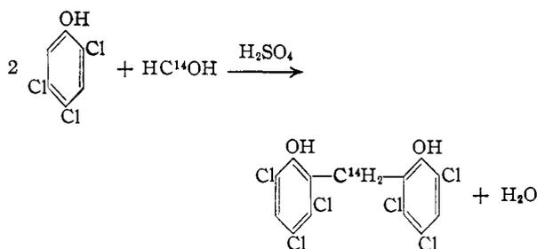
Hexachlorophene- $\text{C}^{14}$  (m.p. 166–167°, cor.) was isolated in a 59.6% over-all chemical yield as two crops, in the second of which 12.5% was recovered with carrier; specific activity (of undiluted product):  $3.58 \times 10^8$  ( $\pm 4.6\%$ ) cts./min./mM.<sup>3</sup>; specific activity of starting formaldehyde- $\text{C}^{14}$ :  $3.52 \times 10^8$  ( $\pm 4.4\%$ ) cts./min./mM.<sup>4</sup>; radiochemical yield:  $60.6 \pm 3.9\%$ .
